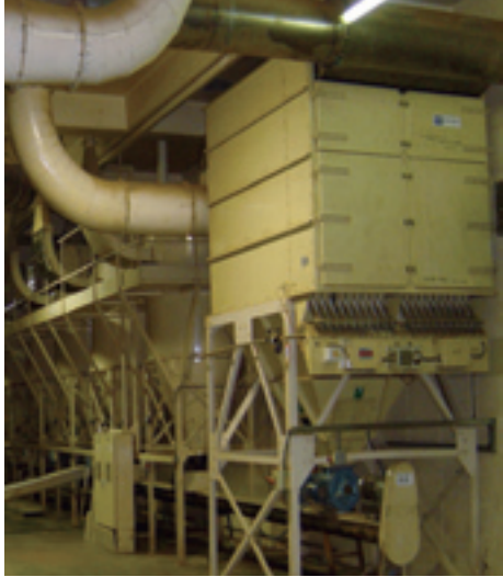
Primary Bag house monitored by Electrodynamic Instrumentation
